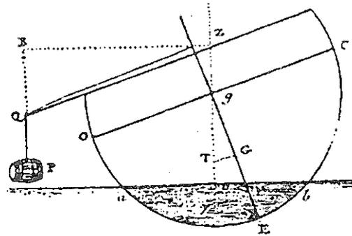
Figure 4: BOUGUER's diagram of an inclining experiment, [2] fig. 55.
